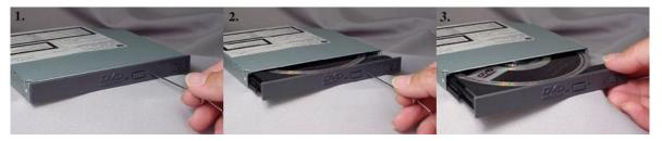
Figure 2.Using Emergency Eject
